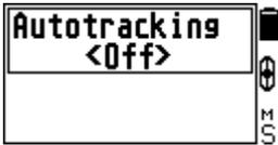
With this setting you can turn on/off automatic tracing of ground balancing change and its correction by the device during operation (for MSF and SSF algorithms only (see below)). When this setting is on, the display shows "A".
