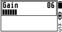
Option allows to regulate searchcoil signal boost for the detection channel (Threshold tone) and identification channel (ST Sensitivity) simultaneously. Such setting may be used in extremely trashy areas, beaches etc, when there is no need in a great search depth, and distinction
