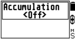
When the storage mode is "off" the display will show only the hodograph of the latest target identified by the device. Once the next target is identified, the previous hodograph is deleted. Mode "2", "3" - the display also saves hodographs from last two or three targets identified by the device. "3" or "2" storage mode is more informative than the "off" mode, and it allows to identify the target more accurately by means of several hodographs resulted from target scanning from different angles.
