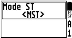
This option allows to change type of sound indication of the ST channel (short tone) between RT, PST and MST. ST is the type of sound indication for the «all metals» operation mode. Threshold detection tone works within the total length of the signal from the object, no matter what the
