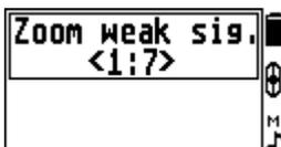
This option was brought to increase capabilities of visual hodographic identification. It allows to increase sizes of weak signal hodographs as well as to evaluate the signal level by the size of the hodographic picture. For instance, setting up 1:2 scale you can increase and thoroughly examine a low-signal hodograph. Scaling 1:7 you can evaluate signal levels in a wider range by the size of the picture respectively.
