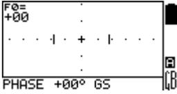
The device automatically initiates the ground balancing (GB) when the searchcoil adaptation is over. The ground balancing is a shift of the ground vector to the horizontal axis. It shall be made in compliance with guidelines of the Ground Balancing chapter. In previous models of the product line the value (degrees) of this shift was equal to the GB value and it was displayed in the bottom left part of the display after the sound indication.
