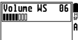
Regulate sound volume weak ST signals from small and deep targets. Low values of this parameter allow to control signal level by the sound volume in wider range of their change. However signals from small and deep objects might be too
