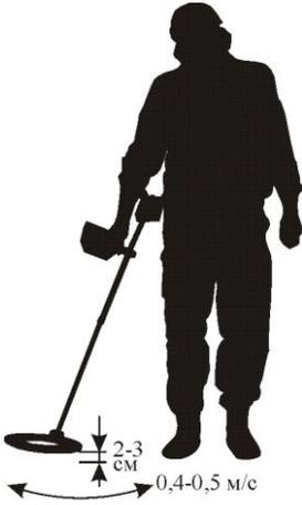
Make additional scanning to detect object type above the center of the object, i.e. on the maximum signal line, keeping distance between the searchcoil and the ground if possible. For the same purpose it is necessary to scan found object in the direction with the least ground relief changes. In this case the ground interference is barely noticeable.
