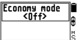
The key feature of this mode is a shift to a low power consumption resulted from the reduction of ECC excitation current. Besides, this mode allows performing ground balancing more accurately when working at the highly mineralized sea beaches. This mode is recommended for trashy areas where high sensitivity is not required.
