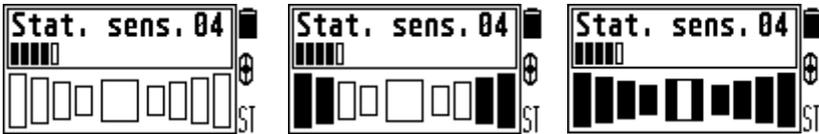
If the signal is too strong and continuous, the target is large and relatively close to the surface. Raise the coil to the level where the target is less responsive and you will be able to detect target contour in the ground by crisscrossed passes.
