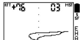
In second case (right picture) it is safe to say that there is a flat iron target under the coil, a piece of iron roof coating, fragment of a kettle, for example.
