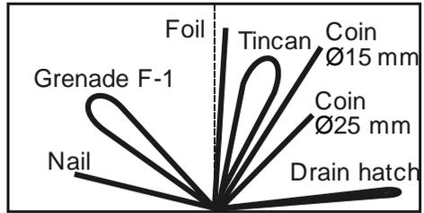
1. Hodographs of small and medium objects made of iron are located in the left half of the screen. In other words, they deflect to the left from the centre of the horizontal axis along the bottom border of the screen.
