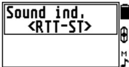
This option allows to change type of sound indication of the RT channel (threshold tone) between RT, RTT and RTM.
