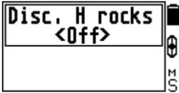
This option allows to turn on/off non-discrimination algorithm of hot rock signal neutralization.
